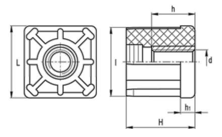
$\begin{array}{ll} d & = M10 \\ h & = 10 \\ H & = 45 \\ h1 & = 10 \\ Internal tube size = 44.0 \\ I & = 44.0 \\ L & = 50 \\ \end{array}$
